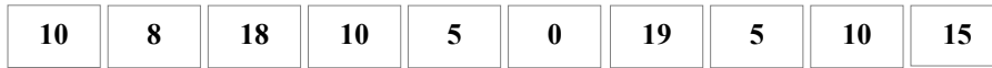
Fig. 1. Chromosome representation for a assignment problem with 10 bugs and 20 available developers. Each chromosome has 10 genes, each of them representing a single bug. Each gene value represents a developer. In this chromosome, developer 10 and developer 5 have been assigned 3 and 2 bugs, respectively.
