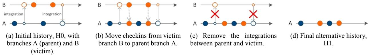
**Figure 5. The steps required to simulate the removal of a branch. In this figure, A is the parent branch, B is the child branch, solid circles represent checkins, hollow circles represent integration checkins between branches. Checkins are colored according to the branch that they were made on in the original history.**
